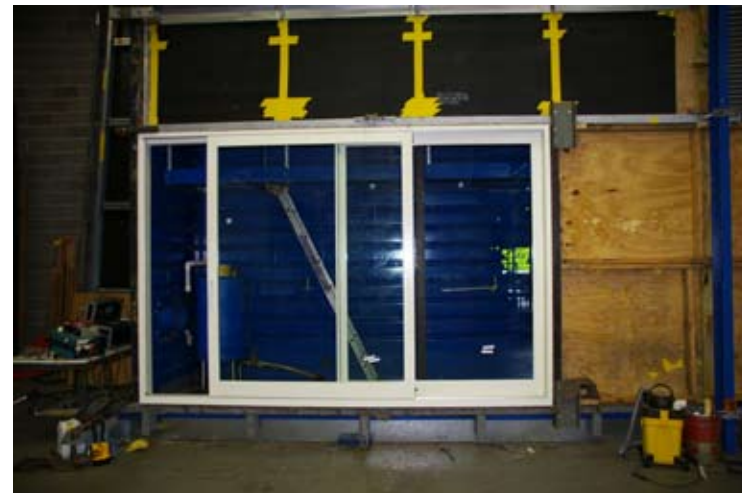
"Lift and Slide" Western Red Cedar Sliding door unit during testing.
