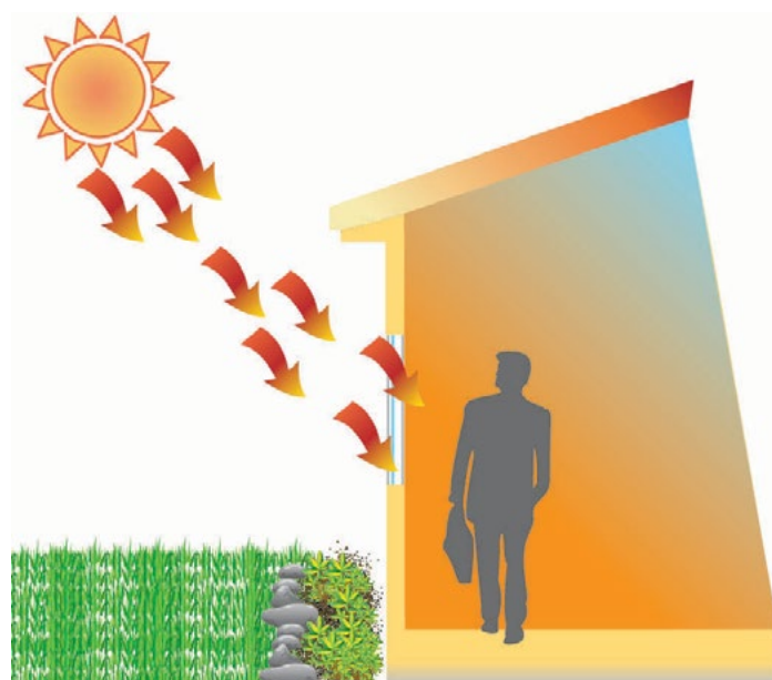
Figure 2.2 Solar Heat Gain Coefficient ( SHGC_w )
